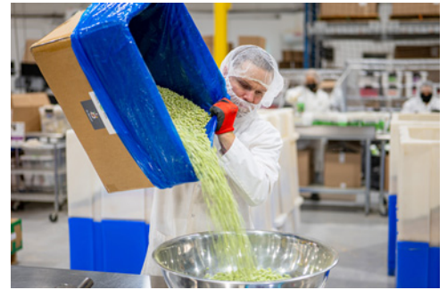
Operators weigh and empty ingredients into bowls which are emptied into a 20 cu ft (0.56 m 3 ) hopper that feeds the Rotary Batch Mixer.
