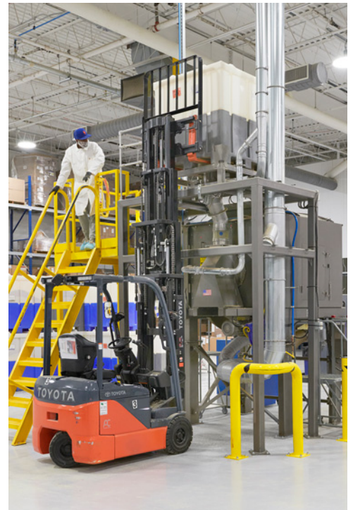
Batched ingredients are gravity discharged from the 20 cu ft (0.56 m 3 ) hopper into the Rotary Batch Mixer of equal capacity.
