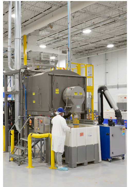
Blended ingredients are transferred from a receiving hopper below the mixer's plug gate discharge valve, into the packaging machine inlet.
