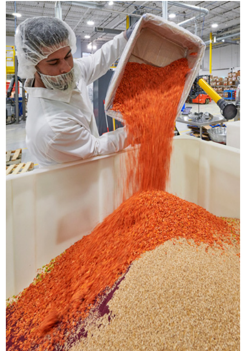
Ingredients are emptied into a 20 cu ft (0.56 m 3 ) hopper that is forklifted into position above the mixer's inlet.
