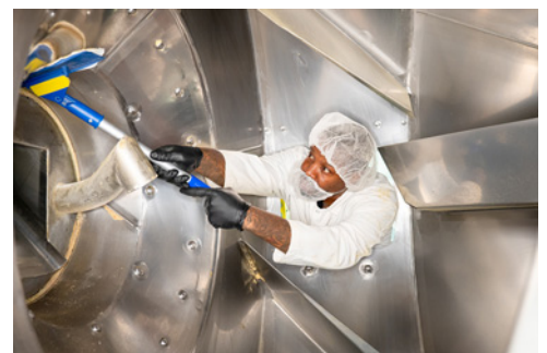
Clean-out doors allow access for cleaning and visual inspection of material contact surfaces.
